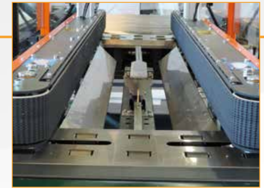
Folding system of bottom flaps (only HM11-TB)
