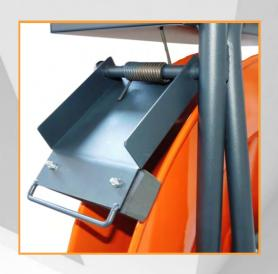
Frame structure reinforced in order to use coils of strapping up to 50Kg. weight.
